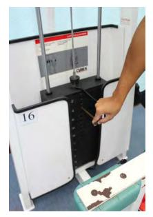
Pull out the handle for adjustment of the weight
