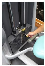
Push the button to pull out the handle for adjustment of the weight
