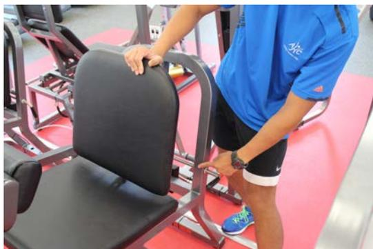
Pull the handle for adjustment of the backrest. Position the backrest so that the knees are aligned with the black pivot point while seated.
