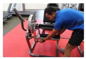
Turn the handle for adjustment of the leg pad length. Position the leg pad so that it is aligned just above the ankle.
