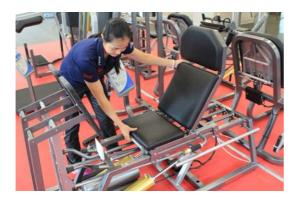
Pull the handle up to adjust the seat length. Position the seat so that the knees make a 90° angle while seated.
